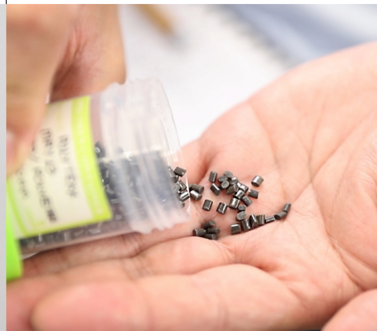
PELLETISE - POLYESTER IS DRIED FURTHER AND THE EXTRUDED INTO PELLETS.
