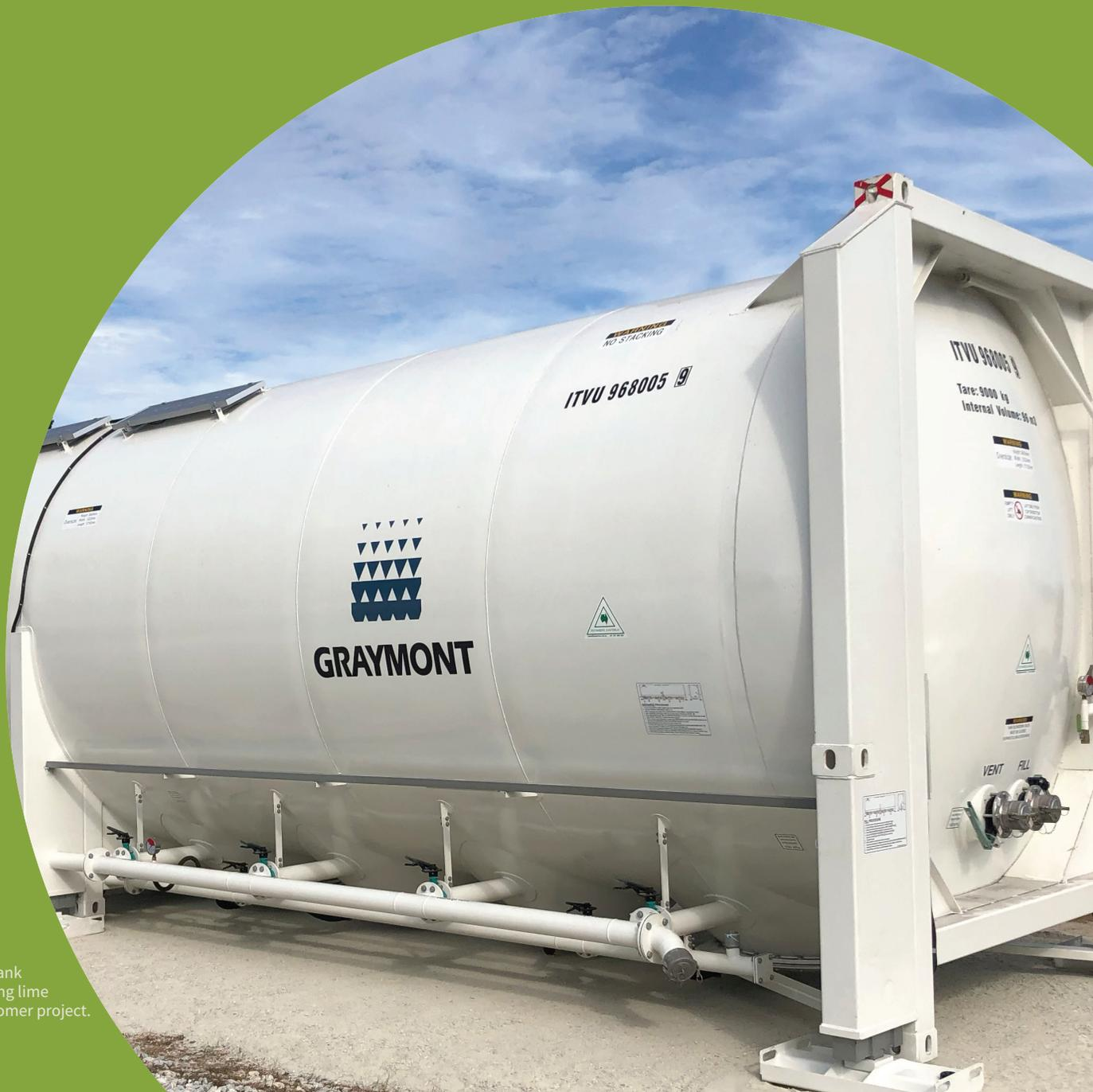
A Graymont ISO tank container providing lime storage for a customer project.
