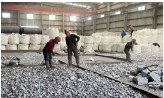
Workers manually crush silicon in Jingang Circular Economy Industrial Park, Ili Prefecture, Xinjiang. Source: Kokodala News via Weixin.
