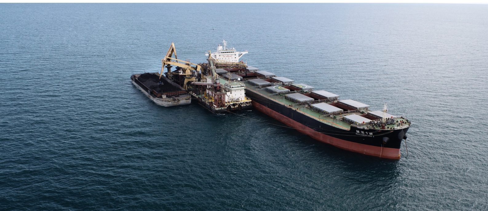
Transhipment of magnetite concentrate from barges to ocean going vessel (OGV) Magsenger 1
